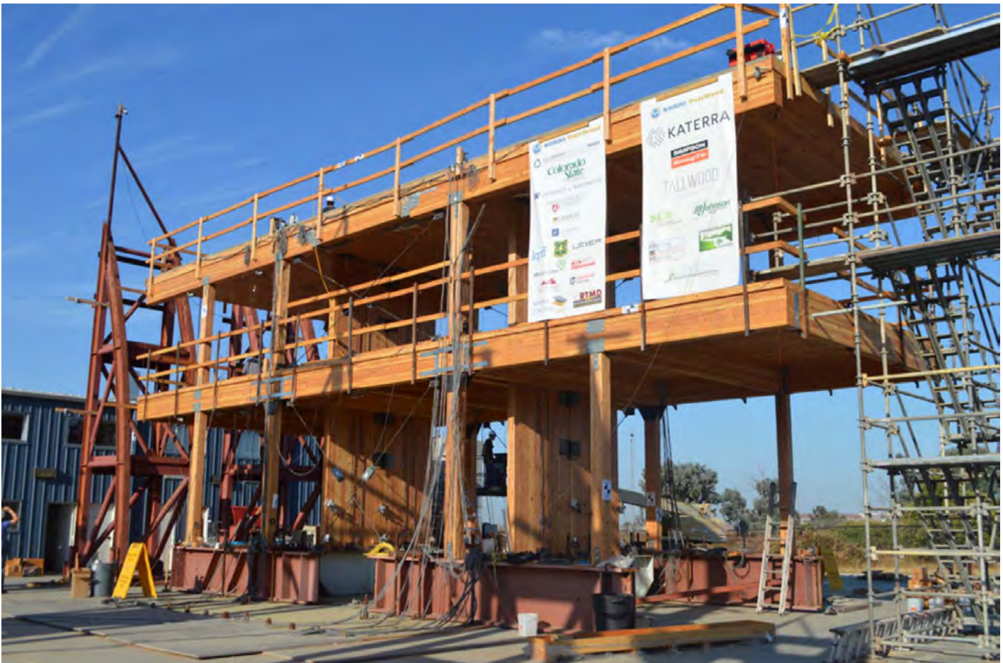
A Resilience-based Seismic Design Methodology for Tall Wood Buildings. Above is the building specimen constructed for full-scale, two-story mass-timber building shaketable tests conducted at the NHERI UC San Diego large outdoor shake table facility. The specimen utilized a lateral force-resisting system consisting of two post-tensioned rocking walls made of cross-laminated timber (CLT) panels.
