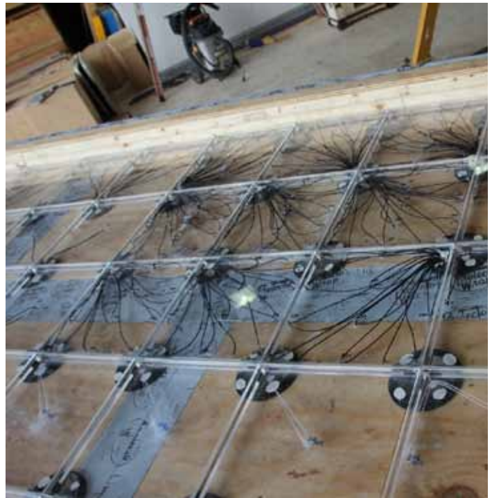
Plastic pavers instrumented with pressure taps.
