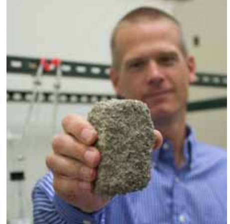
Jason DeJong holds a piece of sandstone-like material created in his lab by the action of microbes on loose sand.
