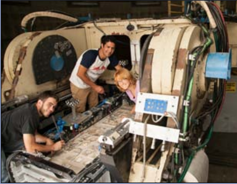
Student researchers work on a centrifuge at the Center for Geotechnical modeling at The University of California at Davis. Current experiments at UC Davis are focusing on soil structure and soil liquefaction.
