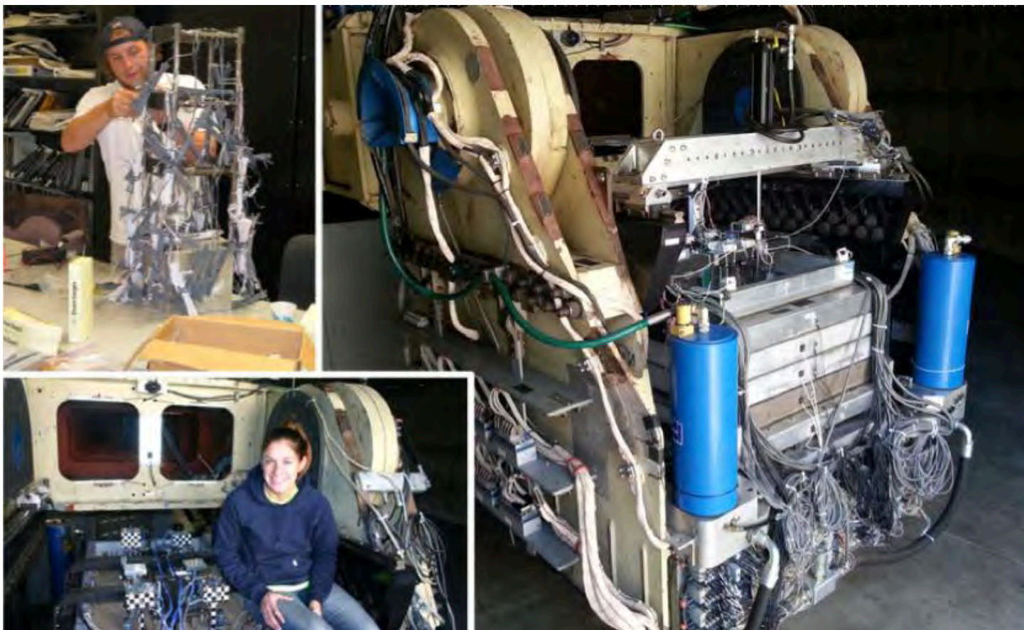
The 9-m centrifuge enables holistic systems-level physical models; e.g., nonlinear multi-story structure-soil-structure interaction (top left insert) and multiple configurations of rocking foundation systems (lower left insert) (Photo: Ross Boulanger, UC Davis).
