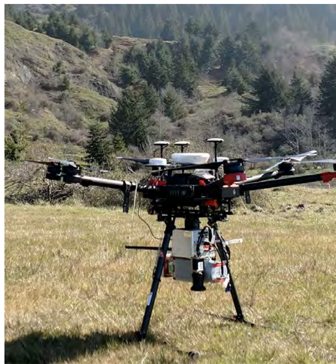
Use of the RAPID facility drone-lidar system to image an active landslide in Oregon (Photo: RAPID Facility).
