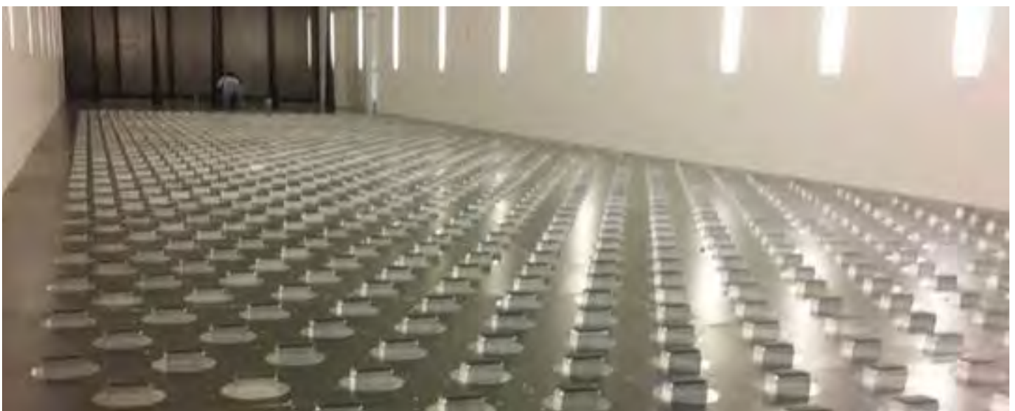
Terraformer for Boundary Layer Analysis at University of Florida NHERI Experimental Facility (Photo: Bernard Brezinski, University of Florida).
