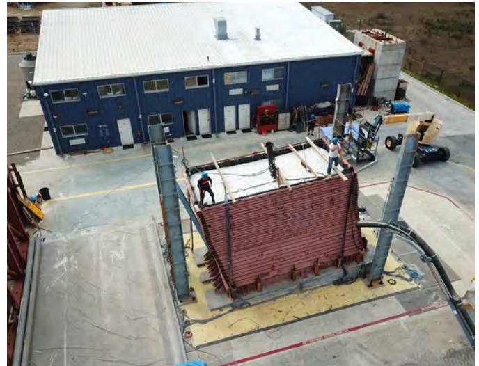
Laminar soil shear box on shake table (Photo: NHERI@UC San Diego).
