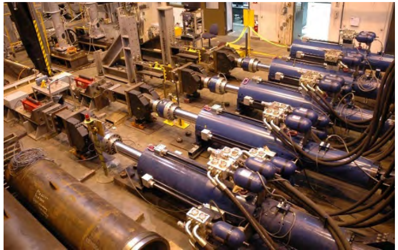
Large-scale damper testbeds for characterization and real-time hybrid simulation of structural systems subjected to wind or earthquake loading (Photo: Jim Ricles, Large-Scale Multi-Directional Hybrid Simulation Testing, Lehigh University).
