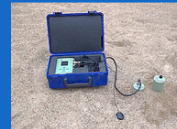
Nanometrics Trillium compact broadband seismometer
