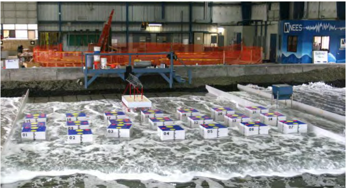
Directional Wave Basin (3D) at the NHERI@OSU Facility (Photo: Dan Cox).
