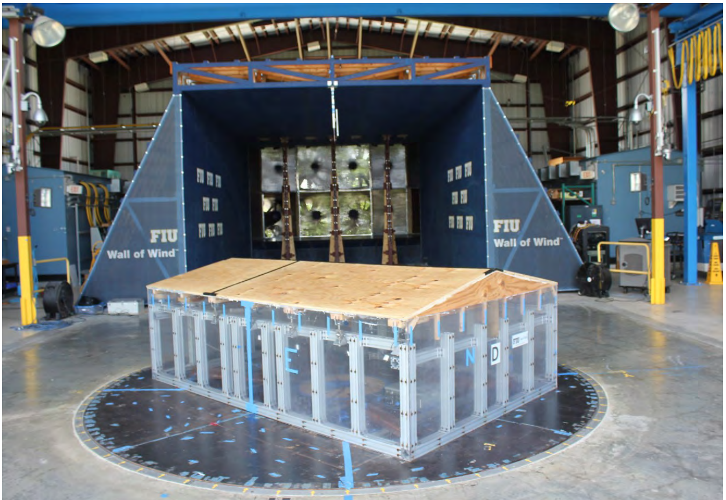
Rotating model for wind effects on small buildings (Photo: Arandom Chowdhury, FIU).
