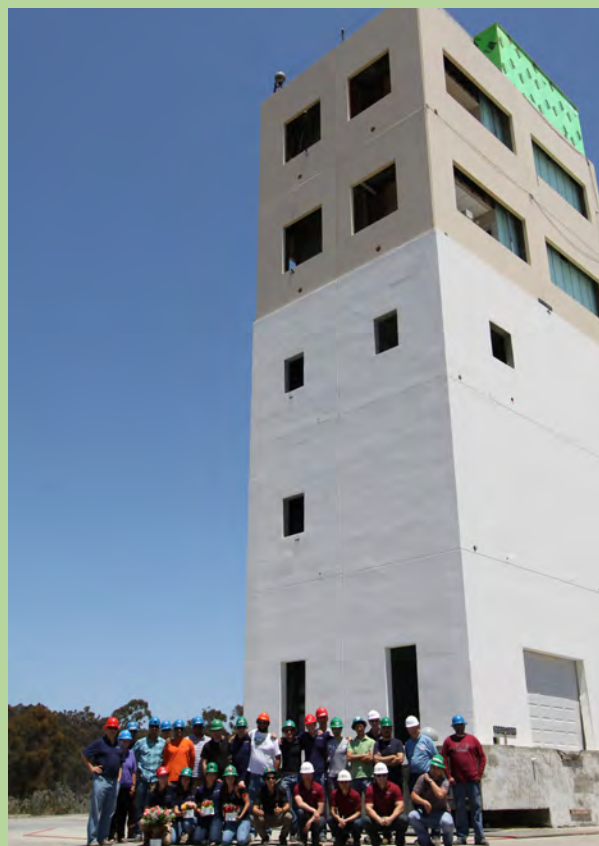
Full-scale structural and nonstructural building system subjected to seismic loading (Photo: NHERI@UC San Diego).
