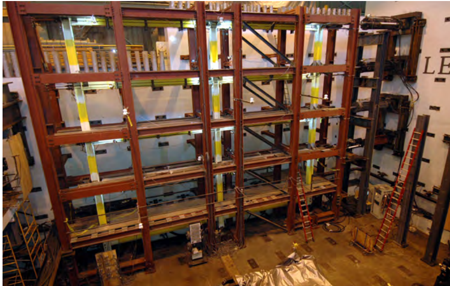
Large-scale hybrid simulation of a self-centering steel moment resisting frame building under simulated earthquake loading. (Photo: Jim Ricles, Large-Scale Multi-Directional Hybrid Simulation Testing, Lehigh University).
