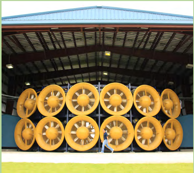
The 12-fan Wall of Wind at Florida International University will enable better engineering against tornadoes, hurricanes and other windstorms.
