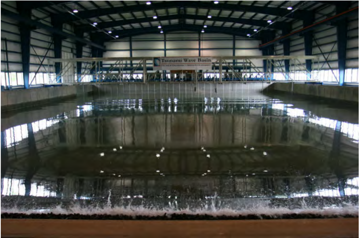
Hinsdale Laboratory three-dimensional wave basin (Photo: Dan Cox, Hinsdale Wave Research Laboratory, Oregon State University).
