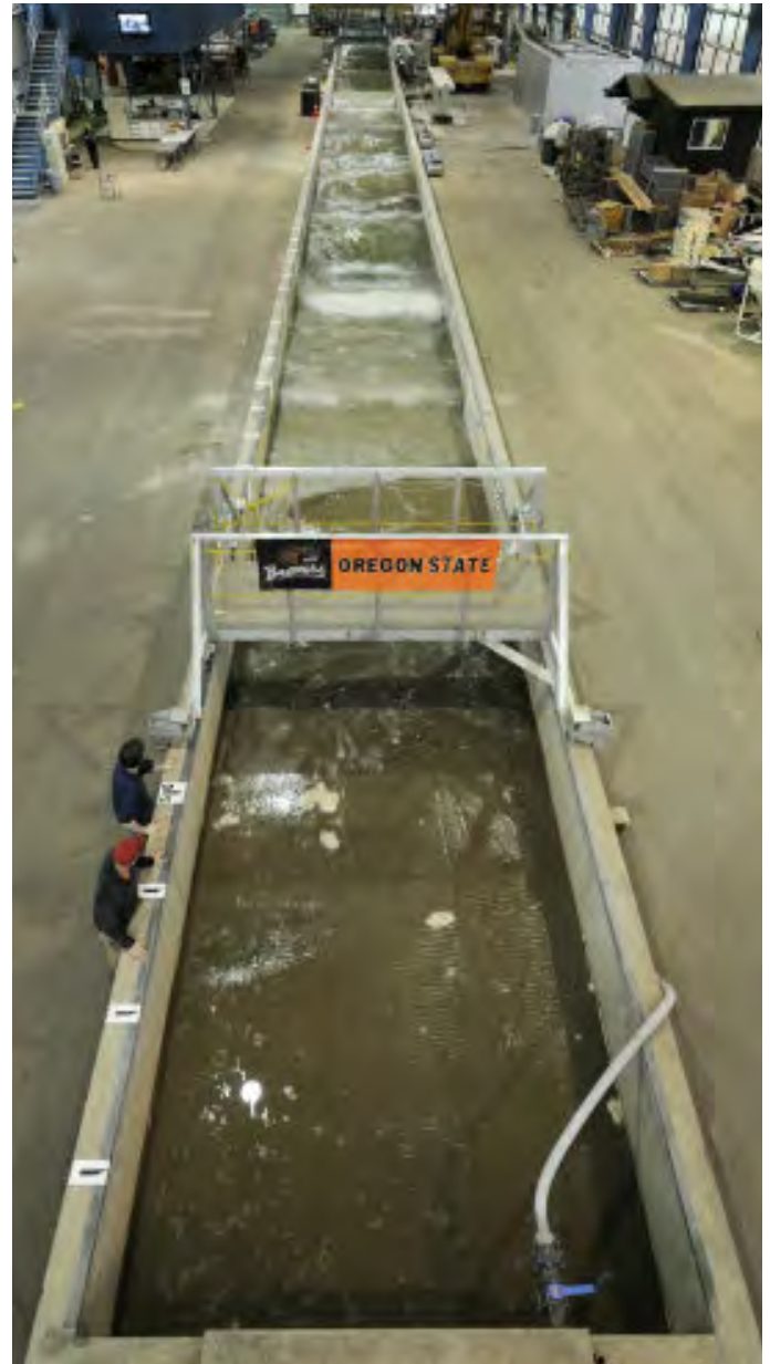
Two-dimensional wave tank with 104m length, 4.6m deep and 2.7m width with wave generation at top of photo (Photo: Dan Cox, Hinsdale Wave Research Laboratory, Oregon State University).
