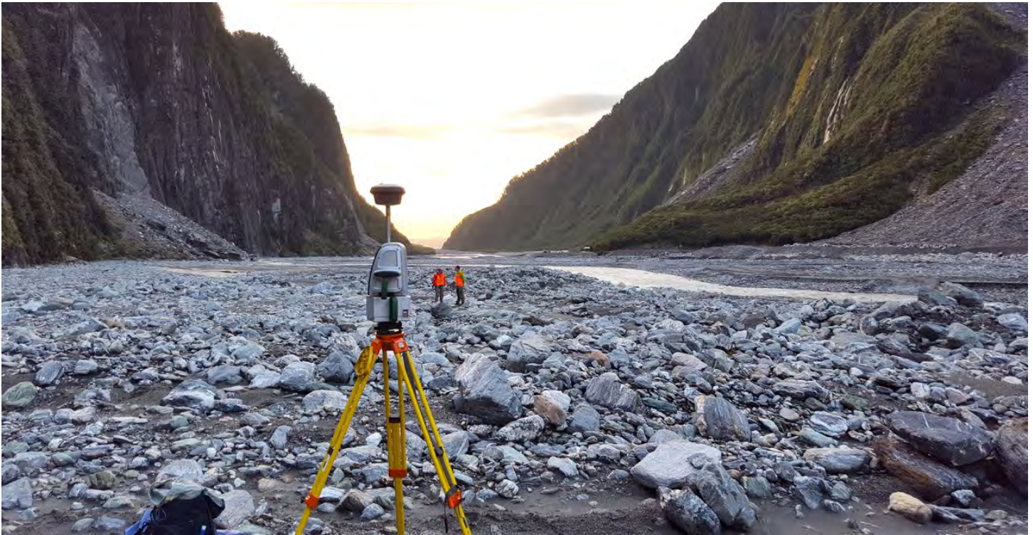
RAPID facility users and staff deployed to the South Island of New Zealand in support of an NSF project to laser scan and characterize precarious rock slopes, which threaten hikers and tourists at the Fox Glacier National Park (Photo: Joseph Wartman, Natural Hazards Reconnaissance Facility, University of Washington).
